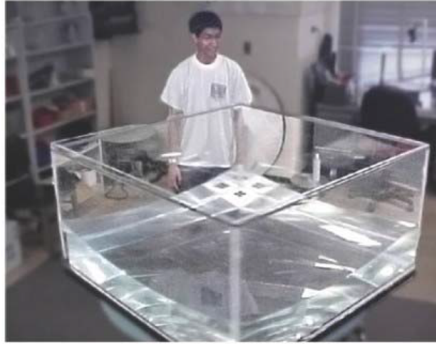
Figure 7: The free surface of a fluid in solid body rotation takes up a parabolic shape, as can be seen in this large square tank of water rotating at 20rpm.
