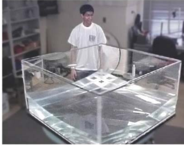
Figure 8: The free surface of a fluid in solid body rotation takes up a parabolic shape, as can be seen in this large square tank of water rotating at 20rpm.
