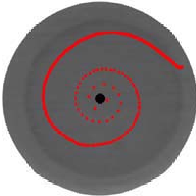
Figure 6: Trajectory of a particle in the rotating frame as it circulates around in the swirling vortex.
