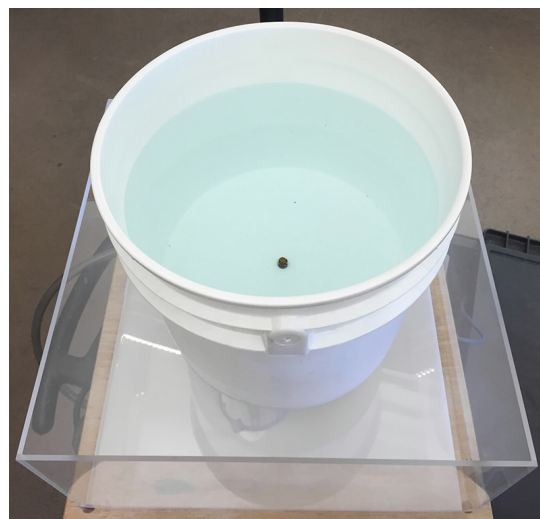
Figure 2: Apparatus used to create a fluid vortex in the laboratory. Water flows out through the hole at the center of a bucket which is rotating about its vertical axis. The bucket drains in to a tank which is seated on a rotating turntable.
